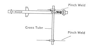
For pulling on one side only, it is best to attach the cross tubes to both rocker panels. Anchor your Dozer to the cross tube. This will prevent undue rolling of the underbody clamps in the pinch weld.
