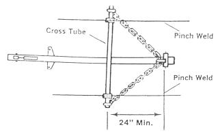
Proper anchoring for a heavy fore and aft pull utilizes the underbody anchoring system as shown here.
