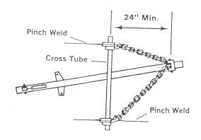
For a diagonal pull, the underbody anchoring system provides attachment to both rocker panels, for better efficiency and less damage. The anchoring loads are spread across both side of the car.
